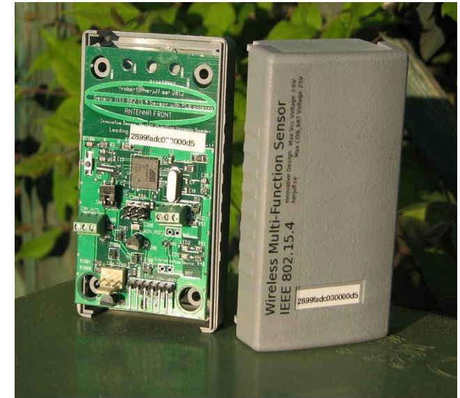
Temperature and Relative Humidity outdoors on garage north wall Broadcasting sensor Node 000c6 with RH-sensor 6131 Powered via solar-charged 12V Lead-acid battery
